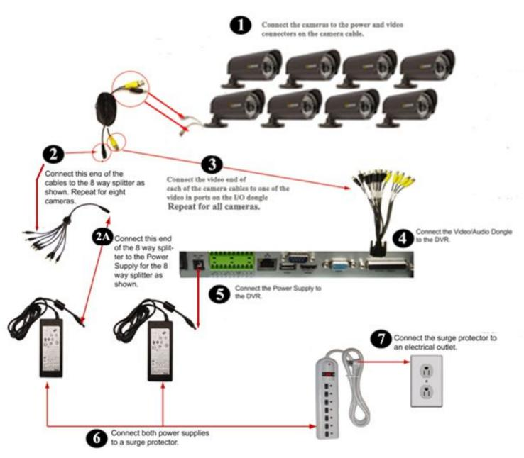
Please note that it is STRONGLY recommended to use a surge protector that is UL-1449 rated. Look for a clamping voltage of 330 or lower, a Joule rating of at least 400 and a response time of 10 nanoseconds or less.
